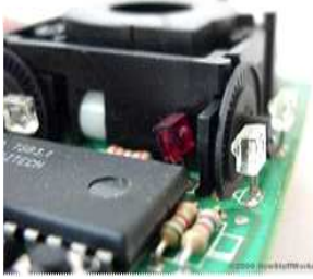
Fig.2.5 A close-up of one of the optical encoders that track mouse motion: There is an infrared LED (clear) on one side of the disk and an infrared sensor (red) on the other.
