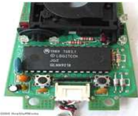
Fig 2.6 The logic section of a mouse is dominated by an encoder chip, a small processor that reads the pulses coming from the infrared sensors and turns them into bytes sent to the computer. You can also see the two buttons that detect clicks (on either side of the
