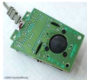
Fig 2.2 The underside of the mouse's logic board: The exposed portion of the ball touches the desktop.
