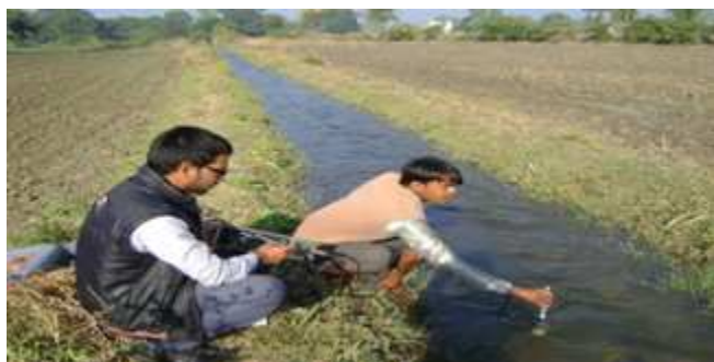
Plate.2 Measurement of canal water flow velocity in head reach
