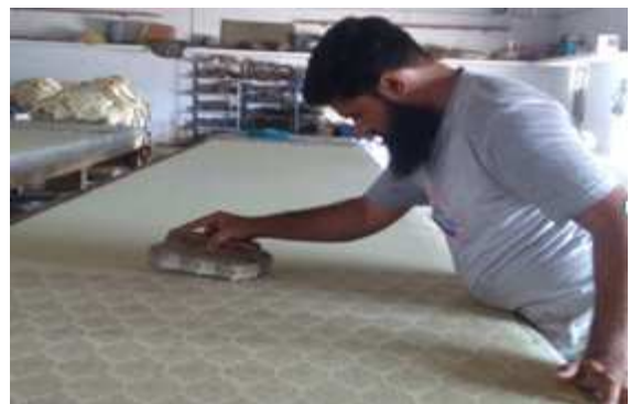
Figure.4 printing the design by using block
